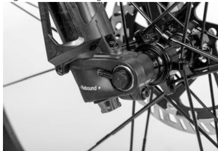
Figure 52: Inserting the breakdown tool
