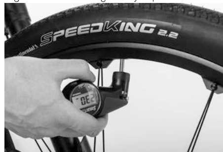
Figure 12: Checking the tyre pressure.
