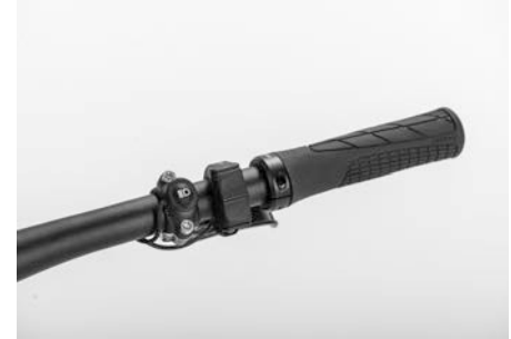
Figure 24: The position of the shifting lever (electronic)
