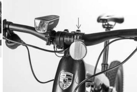
Figure 62: Fitting the front reflector
