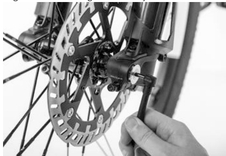
Figure 50: Fitting the safety cover
