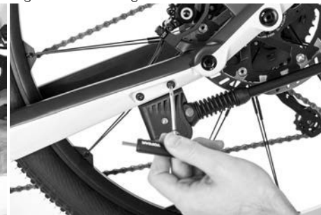
Figure 57: Fitting the stand
