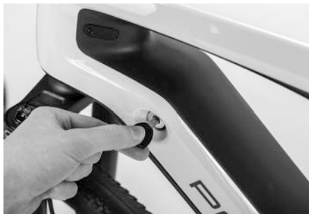
Figure 31: Removing the drive battery
