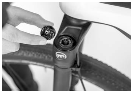
Figure 43: Valve for adjusting the fork pressure.
