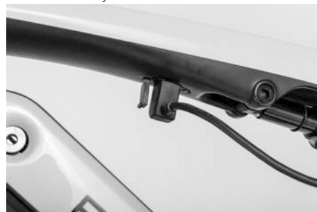
Figure 7: Charger cable connector and drive battery.
