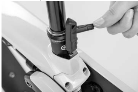
Figure 11: Checking the wedge bolt on the seat post.
