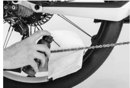
Figure 21: Lubricating the chain
