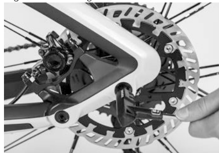
Figure 54: Fitting the rear wheel axle.
