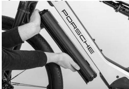
Figure 31: Removing the drive battery
