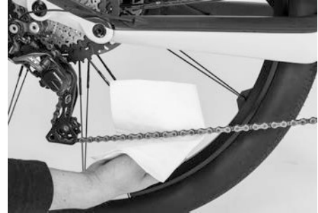
Figure 21: Lubricating the chain
