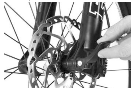
Figure 53: Fitting the Cross front wheel axle system
