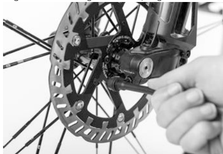
Figure 52: Inserting the breakdown tool
