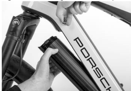
Figure 31: Removing the drive battery
