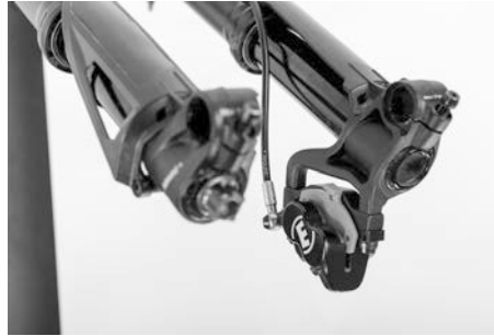
Figure 64: Transport guard for the disc brakes
